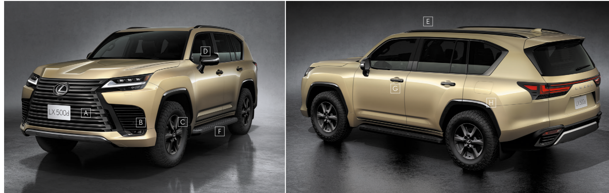
A_Radiator grille / B_Fog lamp cover / C_18-inch aluminum wheels / D_Door mirror / E_Roof rails / F_Door molding / G_Outside door handle / H_Arch molding
